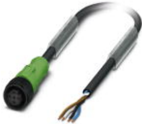
Sensor/Actuator cable, 4-position, PUR halogen-free, Black-gray RAL 7021, Free cable end, on Socket straight M12, A-coded, Cable length: 1.5 m, with plastic knurl
